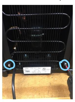
Spread the bottom of cabinet lift up and away from the cooler chassis.
