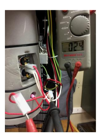
To replace heat band remove the black ties that secure insulation. Once removed pull heat band wires thru the insulation.
