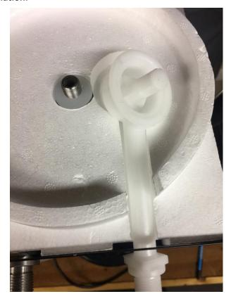
After removing shelf insulation slide waterway to the right and replace with new waterway if necessary
