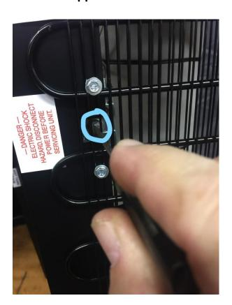
Check wires connected to cold control.
