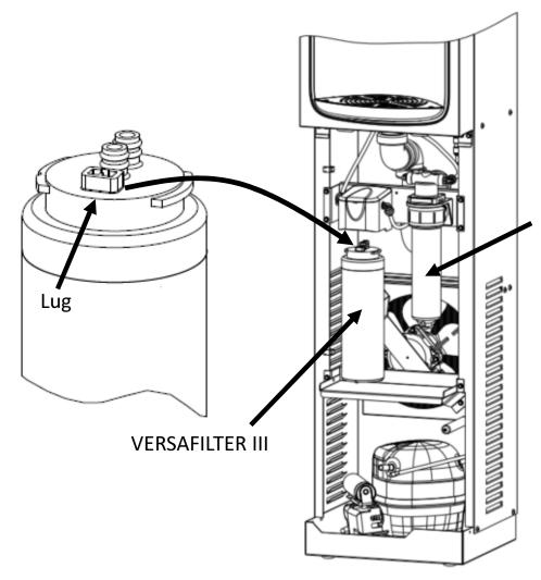
Remedi Filter – shown in Green Filter housing was installed at the factory.
