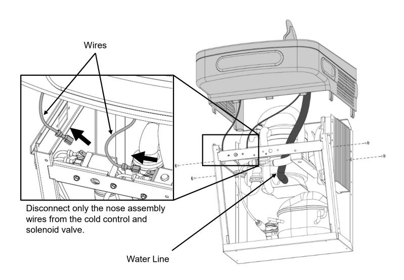
6. After the nose assembly has been removed, cover the two bare terminals with the insulated female spade terminals (provided) for safety.
