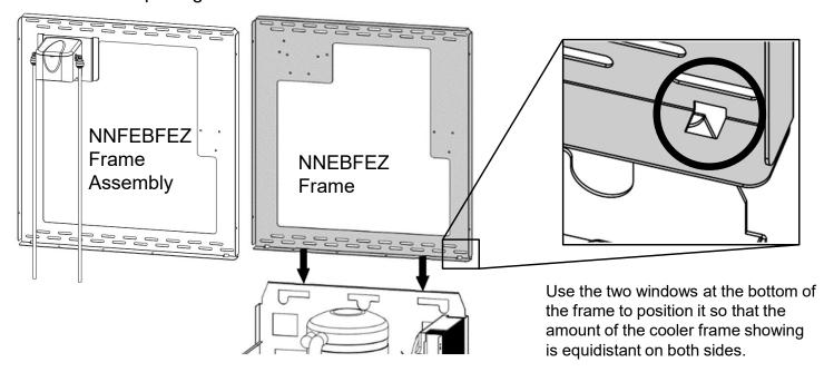
3. Affix the frame to the wall with at least 4 anchors into any appropriate anchor points through the staggered slotted holes. **Be careful to ensure the frame stays centered on the cooler frame.**
