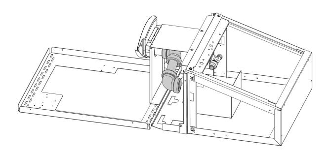
10. Assemble the supplied P-Clip roughly 36" from the grounded plug on the supplied power cord, then secure the P-Clip to the inside surface of the horizontal strut of the fountain frame with a #8 Torx screw.
