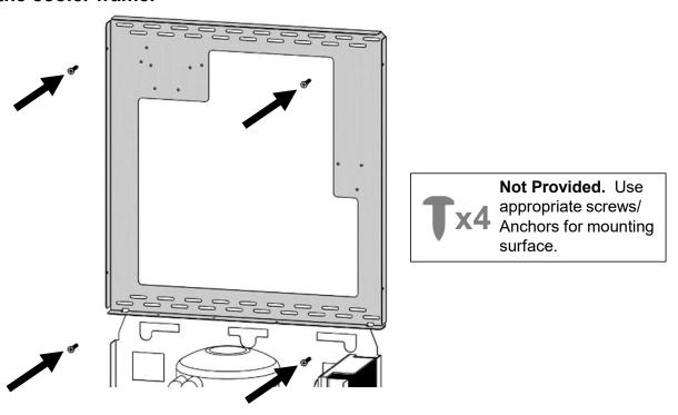
4. Assemble the center bracket to the holes in each of the cooler struts.
