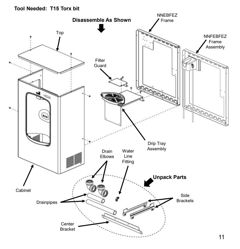
2. Without taking the cooler off the wall, place the retrofit frame against the wall and set it onto the top flange of the cooler frame.
