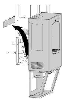
**NOTE:** Ensure that the NNEBFEZ or NNFEBFEZ frame sits on top of the fountain frame. Center the cabinet on the frame as shown on **page 12**. Some extra positioning may be necessary.
