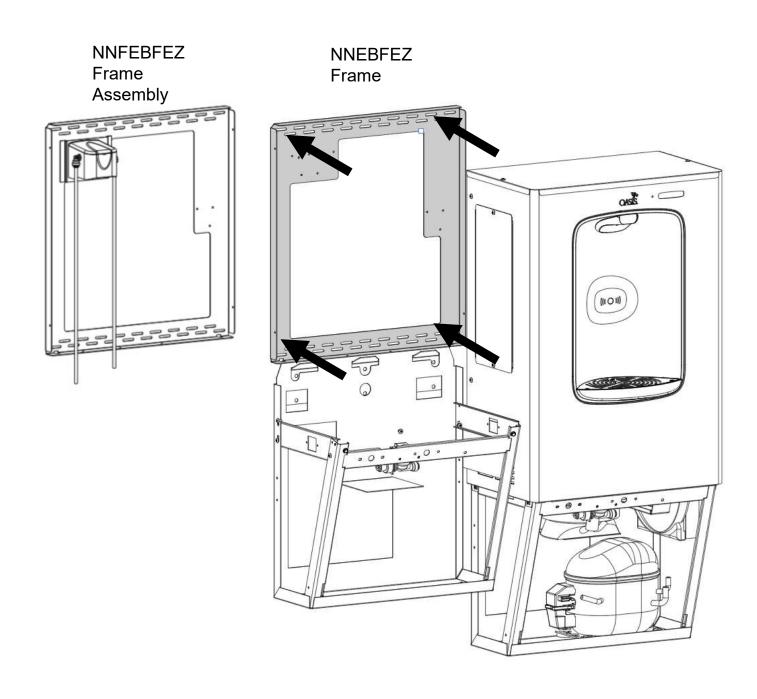
6. Remove the dummy unit from the wall hanger and place it out of the way. Completely assemble a NNEBFEZ to the **refrigerated side first (Refer to pages 11-19)**.
