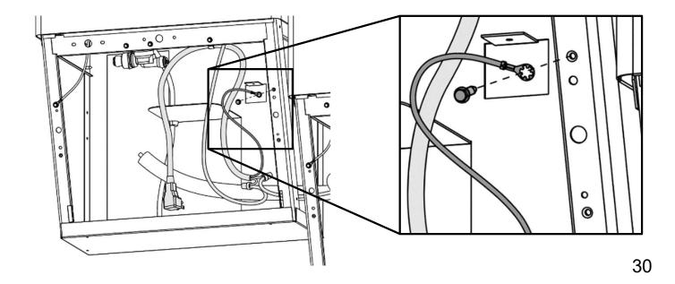
12. Disconnect the IEC connector from the power brick located behind the alcove. Set aside but do not discard the supplied power cord. Do not remove the power brick.
