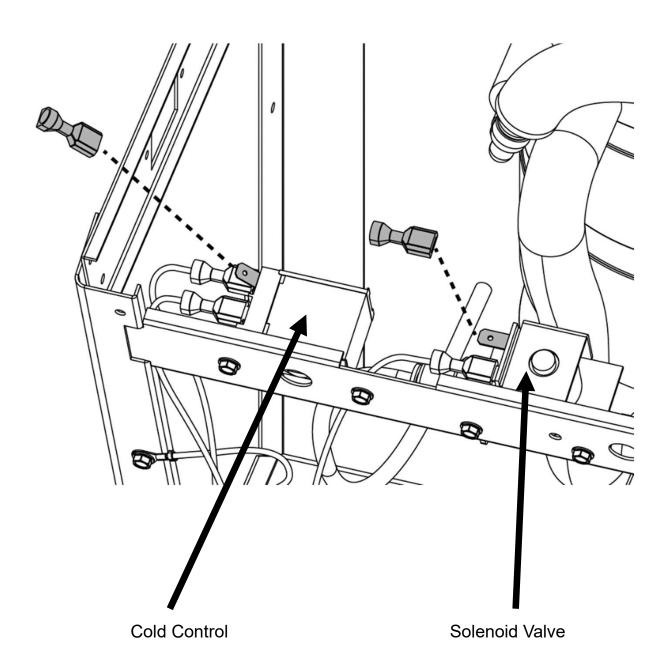
7. Locate the solenoid valve on the Elkay unit. Disconnect both water lines from the solenoid valve. Join the two water lines together using a ½" elbow fitting (provided) (Fig. 7A). For filtered model NNFEBFEZ with the VersaFilter III skip to next page, Section 3A: Step 8.
