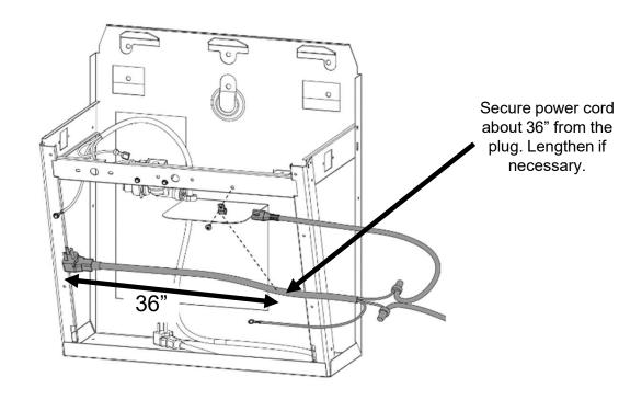
11. Install the ring terminal to the inside vertical strut of the dummy unit with the provided #8 thread cutting hex screw. Screw into one of the empty flared holes of the strut.
