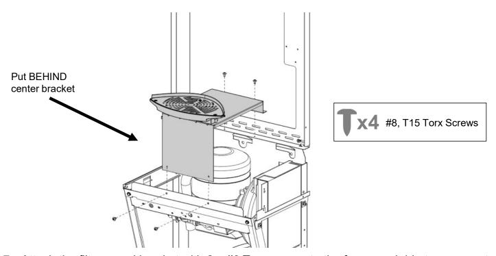
7. Attach the filter guard bracket with 2x, #8 Torx screws to the frame and drip tray support bracket. This bracket helps to prevent the filter cartridge from falling into the cooler unit below during installation or replacement.
