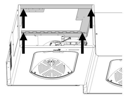
16. After the NNEBFEZ or the Filtered NNFEBFEZ has been hung, the fountain frame may not properly sit back on the wall. Loosen the side screws so that the fountain may rest against the wall, then re-tighten the side screws.
