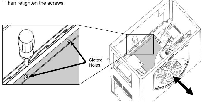
12. Once the wrapper has been installed, loosen the side bracket mounting screws until the bracket can be slid up and down. Adjust the bracket until the mounting hole screws through the slot and then drive in one of the #8 Torx screws and then tighten the two #10 mounting screws.
