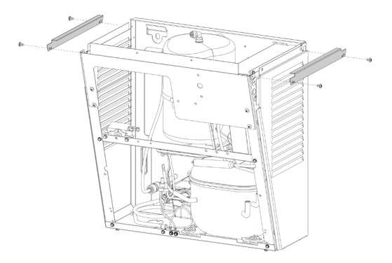
Align each bracket as shown. Use the clearance hole to attach the screw in the cooler strut (away from the wall) and use the slot to attach the bracket in the rear (closer to wall).
