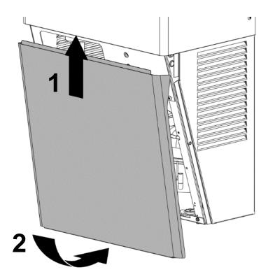
Complete the installation by installing the Top and filter access panels.
