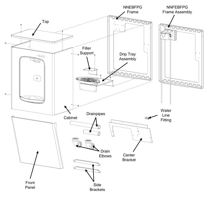
2. Assemble the center bracket to the holes in each of the cooler struts with 4x T15 Torx screws.
