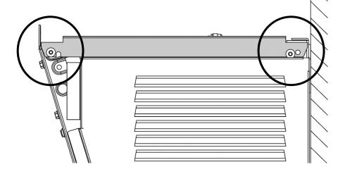
4. Without taking the cooler off the wall, place the retrofit frame against the wall and set it onto the top flange of the cooler frame.
