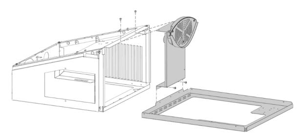
9. Remove the top panel from the NNEBFPG or NNFEBFPG wrapper assembly and lay the wrapper over the assembled frame and drip tray. Secure with 4x T15 Torx screws provided. Refer to **page 17.**
