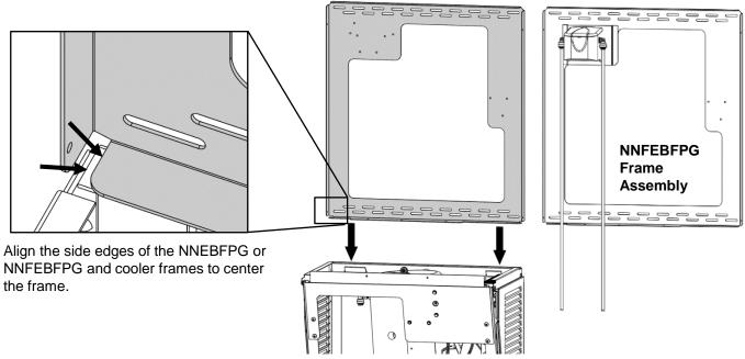
5. Affix the frame to the wall with at least 4 anchors into any appropriate anchor points through the staggered slotted holes. Be careful to ensure the frame stays centered on the cooler frame.
