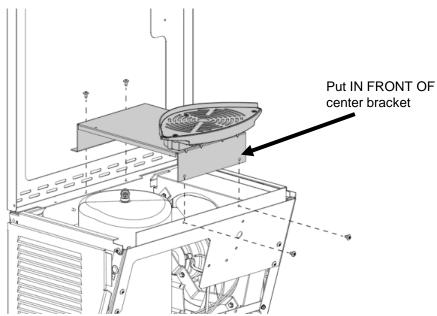
7. Attach the filter support bracket with 2x T15 Torx screws to the frame and drip tray support bracket. This bracket helps to prevent the filter cartridge from falling into the cooler unit below during installation or replacement.
