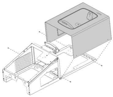
10. Carefully lift the assembled dummy unit by taking hold of the fountain frame and NNEBFPG or NNFEBFPG kit. Hang the assembly back on the vacant wall hanging bracket.
