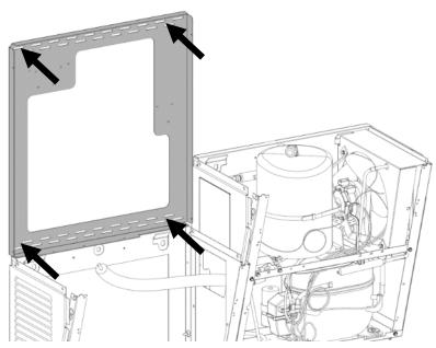
5. After the holes have been drilled, remove the dummy unit from the wall but **do not remove** the hanging bracket.
