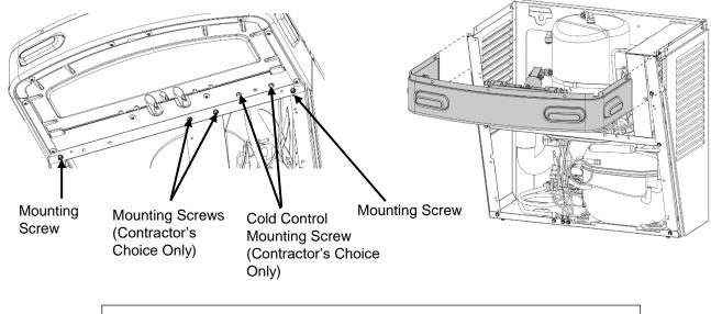
**CONTRACTOR'S CHOICE MODEL:** The cold control will be unsupported at this point. Secure it as necessary and ensure the cap tube does not kink.
