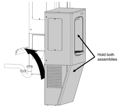
11. Ensure that the frame and fountain are flat against the wall and install your 4 chosen wall anchors (not supplied) to secure the NNEBFPG frame or the NNFEBFPG frame assembly to the wall. Ensure that the NN(F)EBFPG frame remains centered on the dummy unit frame. **Refer to page 13.**
