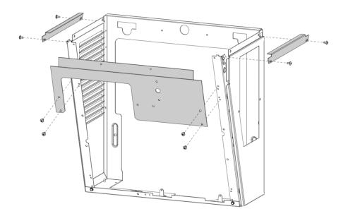
8. Lay the dummy unit on the floor and set the NNEBFPG frame or the NNFEBFPG frame assembly onto the unit and then install the drip tray bracket assembly with the T15 Torx screws provided. Refer to **page 14.**
