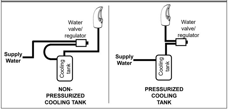
1. With the cooler top removed, find the tube going from the cooling tank outlet to the valve. The TEE fitting (supplied) will need to connect between the cooling tank and valve.
