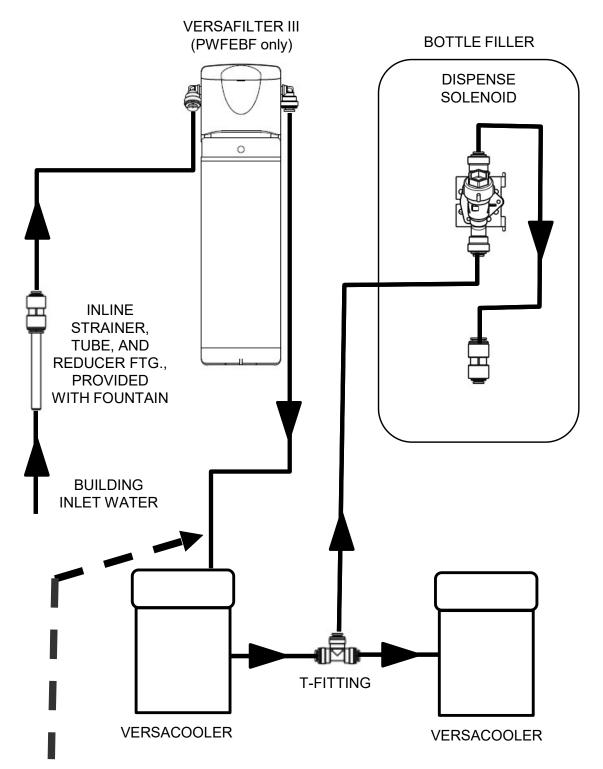
**IMPORTANT:** Flush filters before connecting water line to VersaCooler. PWFEBF only.
