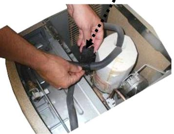
3. Pull back insulation and cut the copper tube with a tubing cutter. Cut where there is at least 1 inch of *straight* tubing on each side of the cut.
