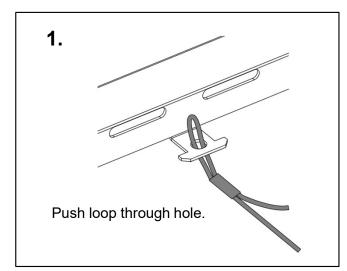
Attach the tether line assembled to the bottle filler dispense bracket to the cleat on the
