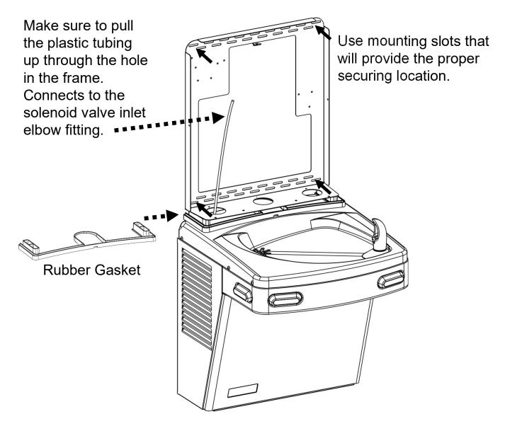
3. Secure frame to the wall with fasteners (not provided). Pull plastic tubing up through the hole in the frame.
