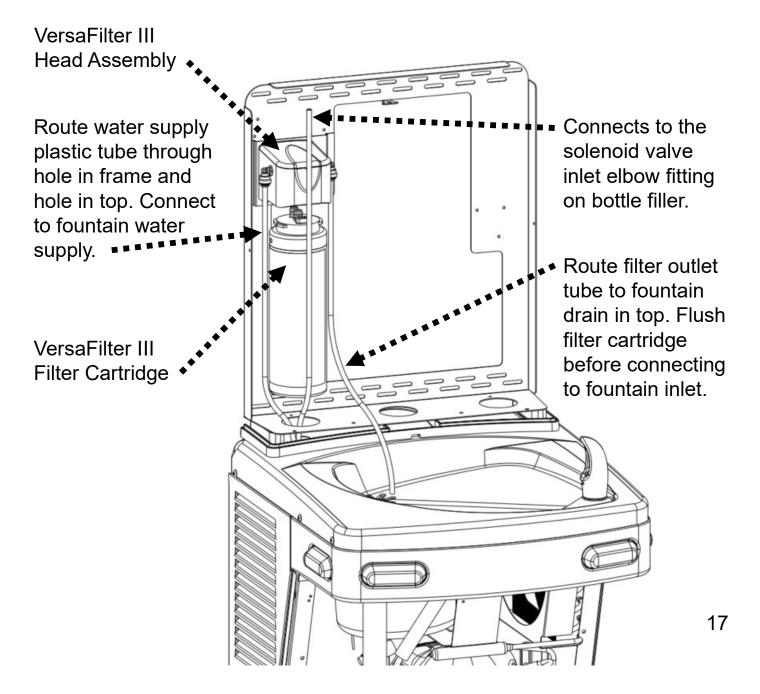
1. Slide sponge tubing insulation over water line. Connect the tubing to the INLET of the solenoid valve elbow fitting on the back of the Hands-free VersaFiller assembly.
