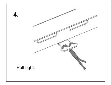
The tether keeps the bottle filler secured to the frame when changing the filter. Make sure the tether is installed properly to avoid accidental damage to the unit.
