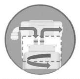
When the <u>Versafilter</u> III is inserted in the filter head and given a ¼ turn, the filter will lock into place and opens the waterway to allow flow into and out of the filter
