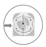
When in the "OFF" position the water inlet is blocked by the filter head.
