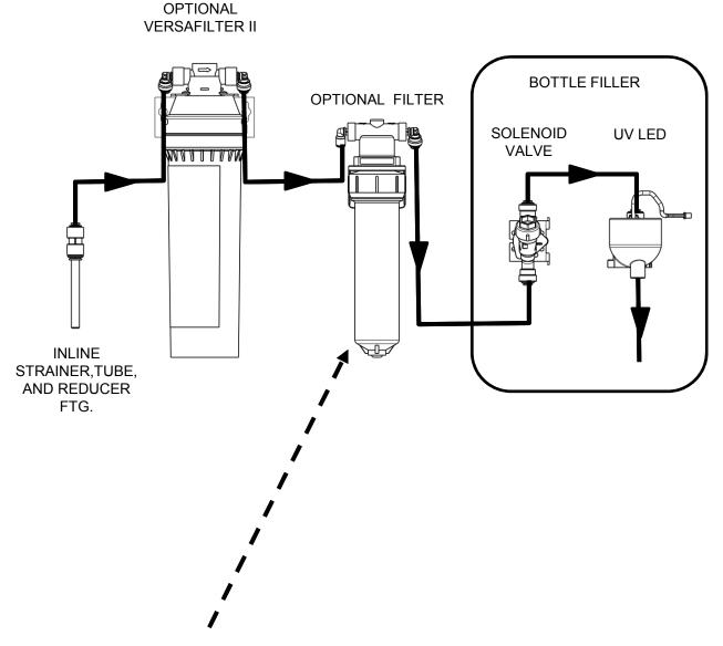
**IMPORTANT:** When replacing filter cartridge, depressurize water lines prior removal of filter housing from the quarter turn filter head assembly.
