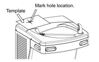
Remove top from cooler by removing six, #15 torx head screws on sides of top.
