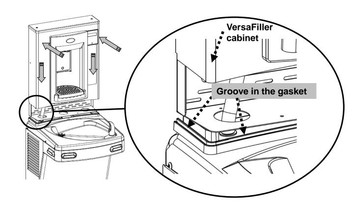
See next page to secure Bottle Filler assembly to frame with torx screws.
