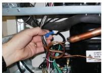
Next, insert end of tube into fitting.
