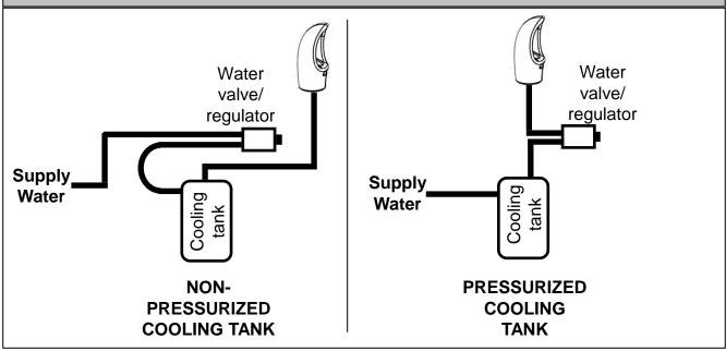
With the cooler top removed, find the tube going from the cooling tank outlet to the valve. The TEE fitting (supplied) will need to connect between the cooling tank and valve.
