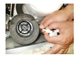
3. Using the 38" piece of tubing provided, cut 6" and install it on the end of the TEE. Install the remaining tubing onto the branch of the TEE. Connect the other end of the TEE to the tank outlet tubing (tube that was disconnected from the elbow).
