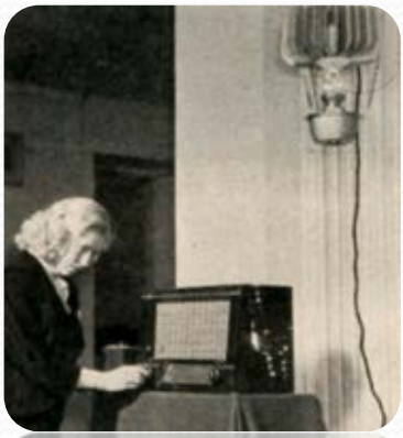
Oil burning lamp powering a radio using a TE generator (1948)
